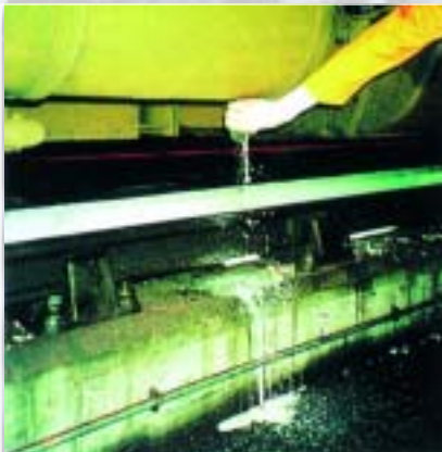
Condensate collected in the main receiver of a locomotive stood overnight in the sidings.
